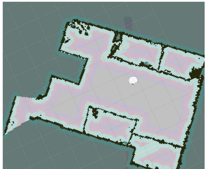
Fig. 8: Global Costmap With Obstacle Layer of 0.3m
