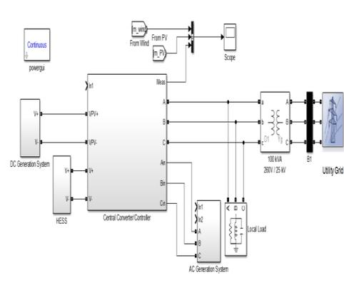
Fig. 4. Outer layout of the proposed system in Simulink
