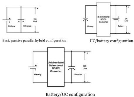
Fig. 3. General Layout of HESS
