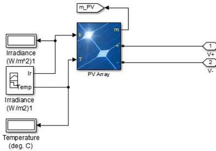
Fig. 6. DC generation layouts in Simulink(PV Solar Panels)
