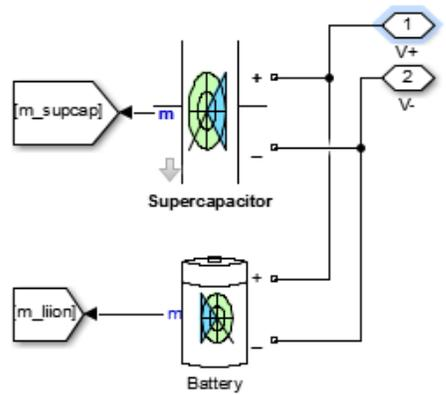
Fig. 7. HESS layouts in Simulink(Battery and Supercapacitor)
